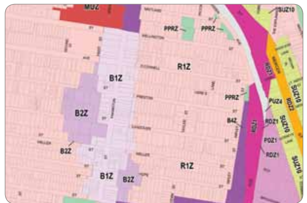
Figure 2. A zoning plan for an urban area, outlining the different zones that apply to each piece of land. Source: Department of Planning and Community Development (DPCD) web site, November 2010.
